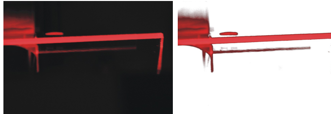
Figure 6-2: 2db/cm loss waveguide with black removed
